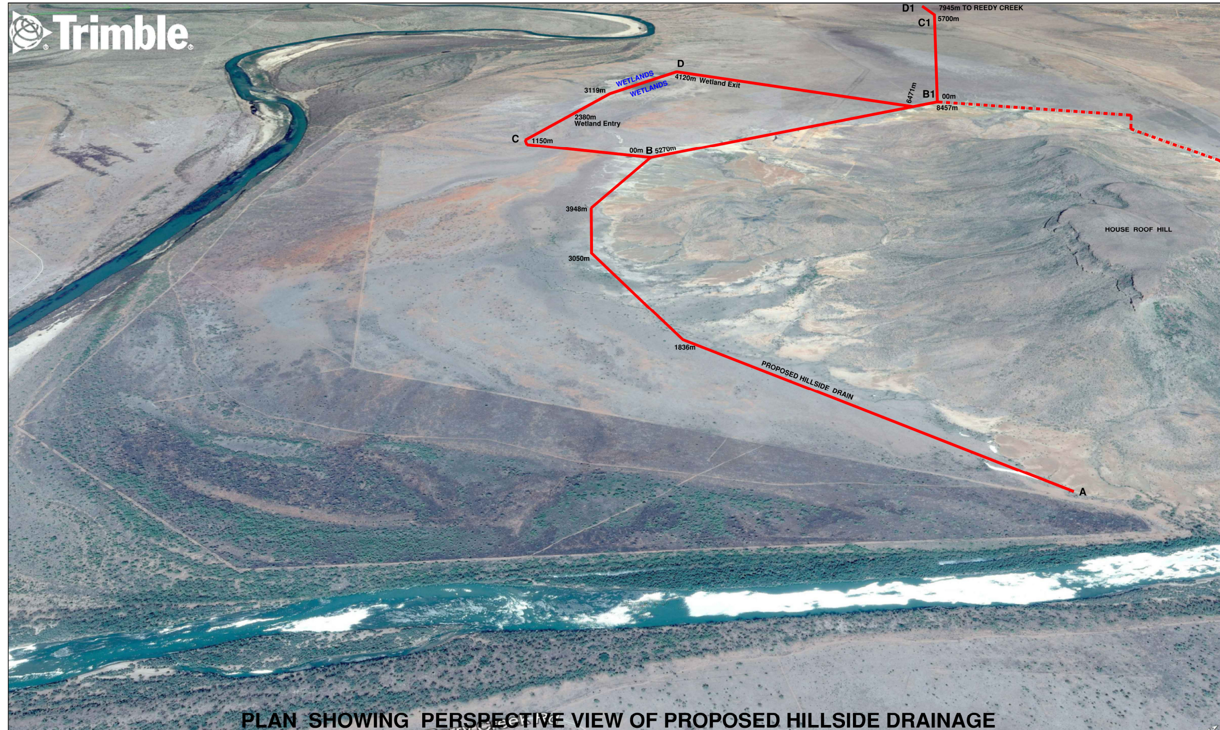
Figure 7 - Hillside drainage for flood water management
