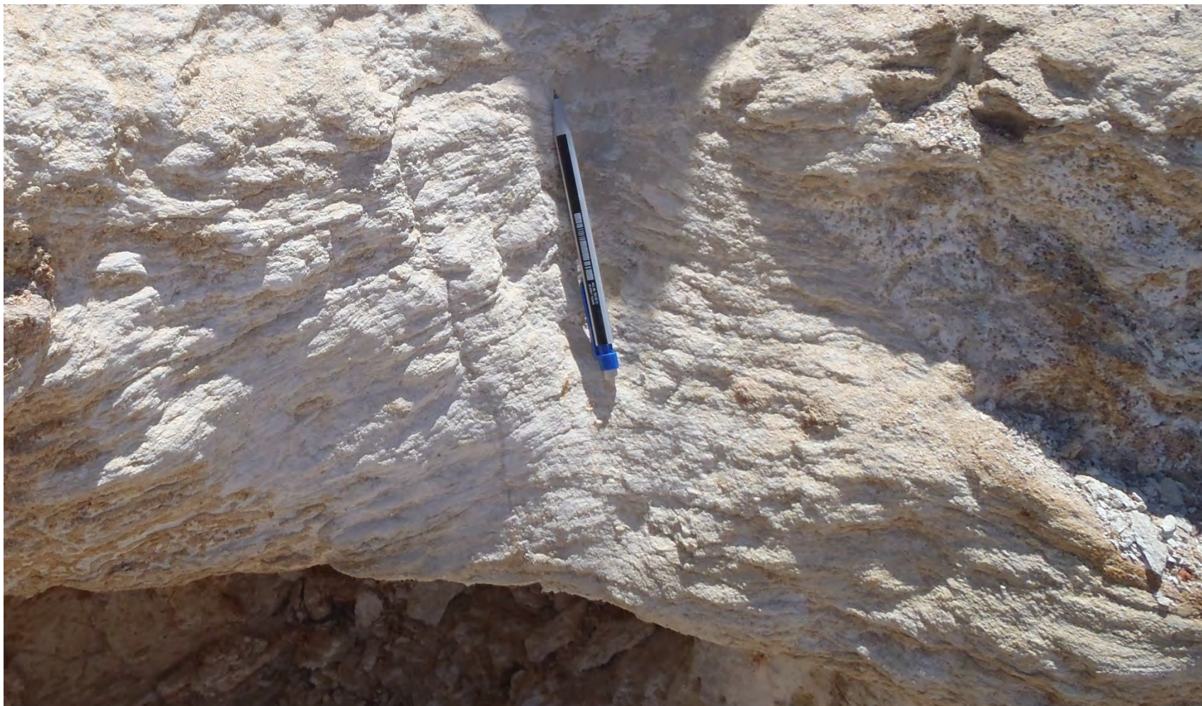
PLATE 3 – Typical Rock Schistosity
