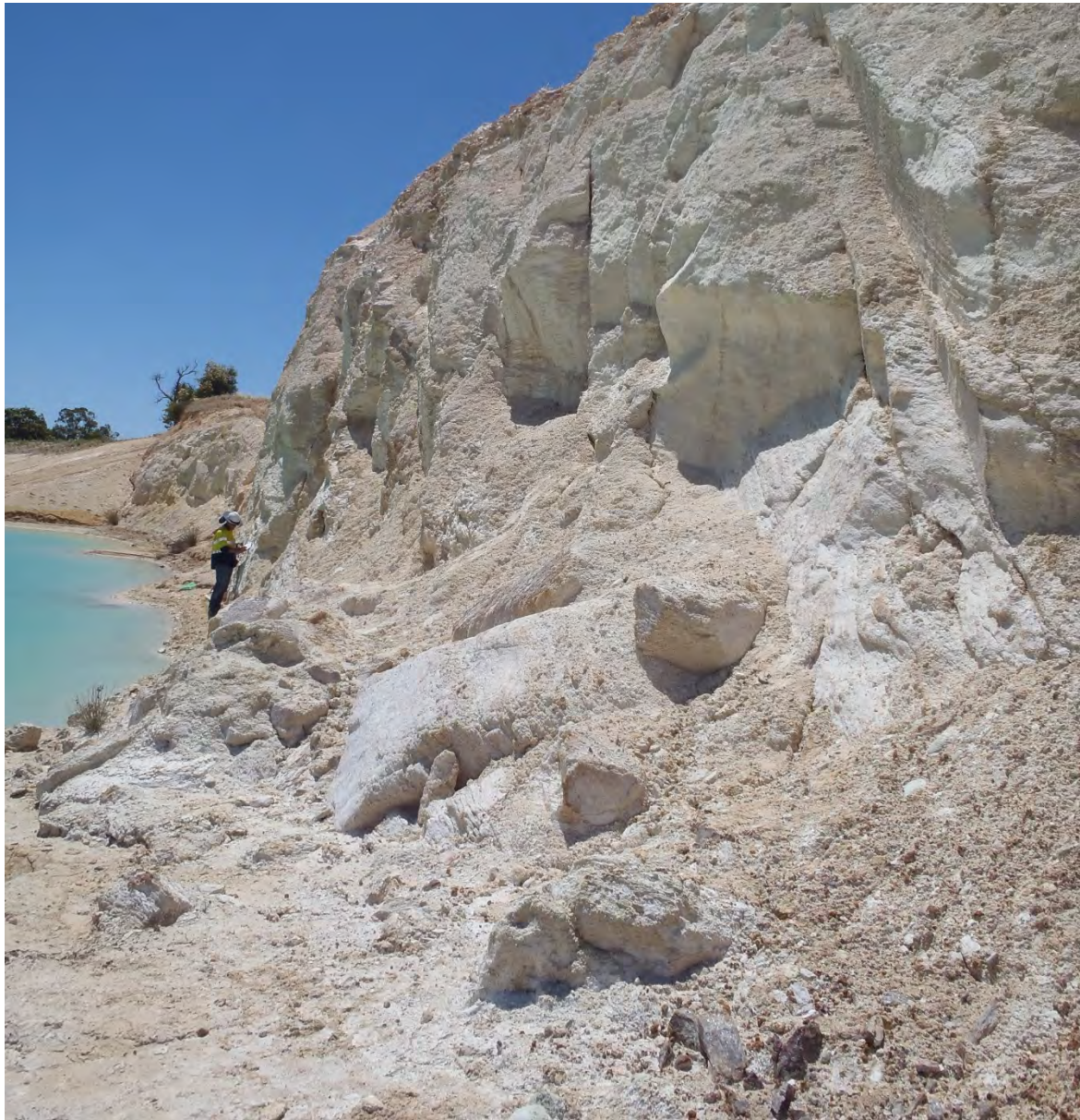
PLATE 4 – Open Jointing and Slope Debris at Base of Slope Observed in Exposure 2
