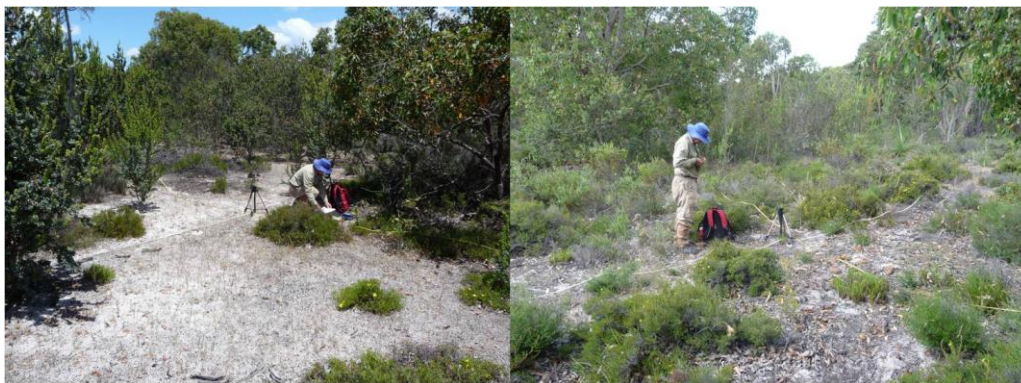
Plate 3. Examples of field assessment of shot point locations with central location marked by the tripod, established using a hand-held GPS, with 10 m of measuring tapes crossing over this central point.
