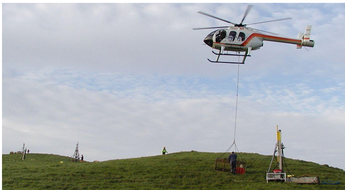
Plate 2. Four heliportable shothole drills supported by one helicopter. Taranaki, New Zealand, 2004. Image courtesy T. Grocke.
