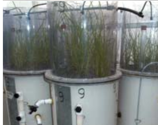
Advanced bioretention columns for testing the performance of anaerobic zones in nitrate removal, and for determining optimum filter characteristic
