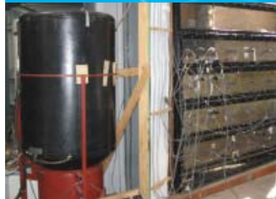
Experimental rig for testing resistance of filter-media to long-term sediment loads
