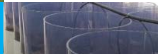
Laboratory columns set up in greenhouse for column experiments
