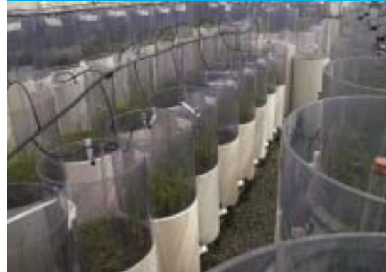
Large bioretention columns for testing design and operating conditions
