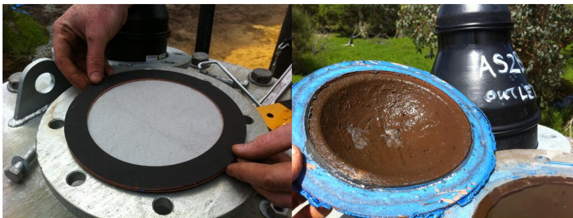
Figure 10: Active System Filter, pre filtration (left) and post “fouled” (right)
