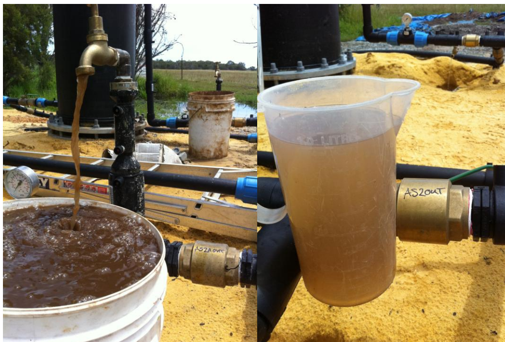
Figure 9: Flow collection point from an active system filter and 1 L beaker used for flow measurement
