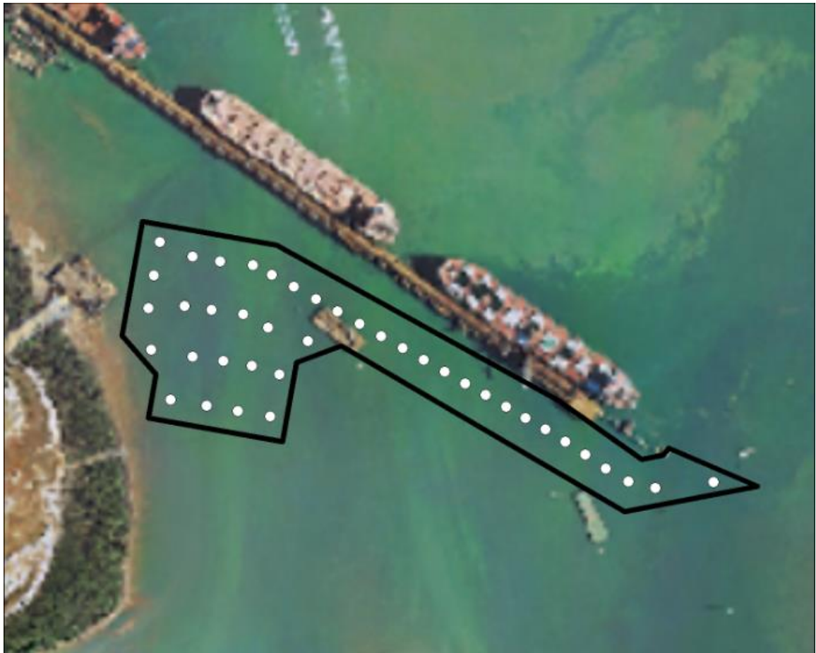
Figure 3-4: Proposed dredge footprint with spill locations as implemented in the sediment plume model.
