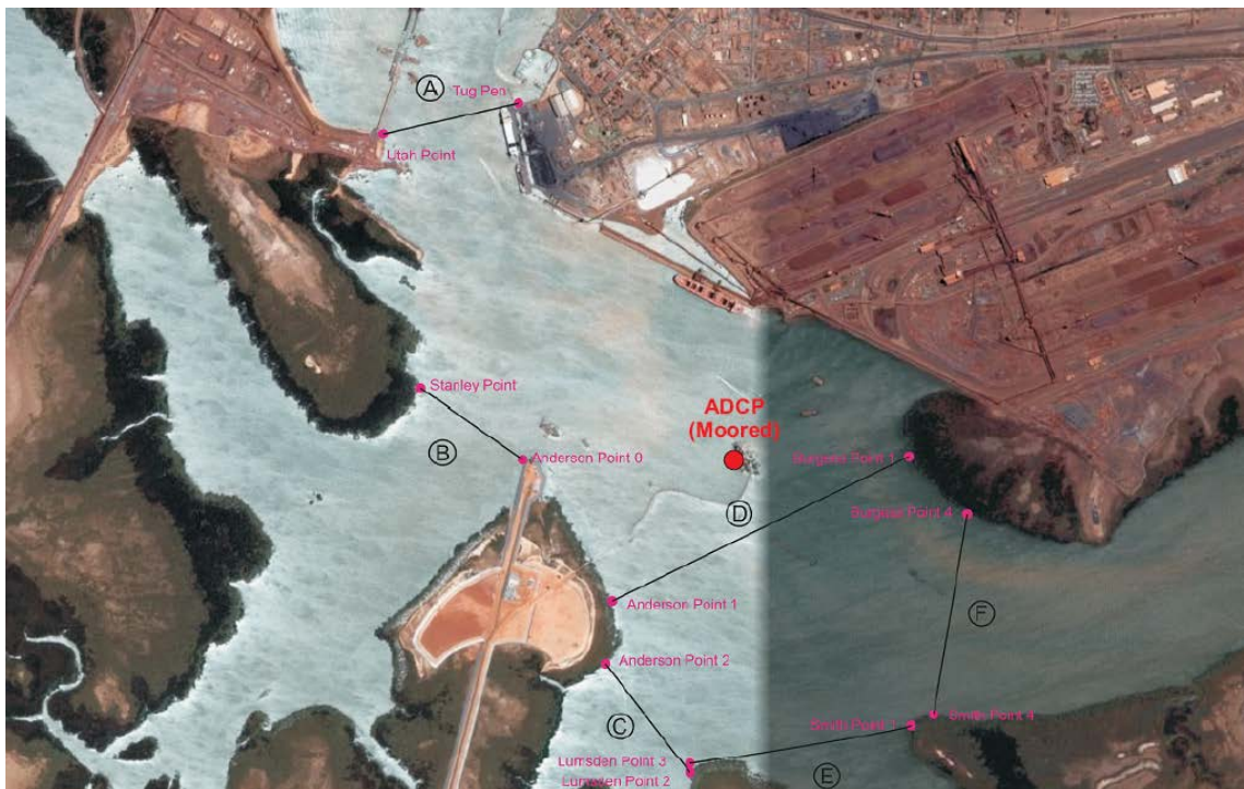
Figure 3- 1: Locations of measurement data (ADCP transects and moored ADCP) for validation
