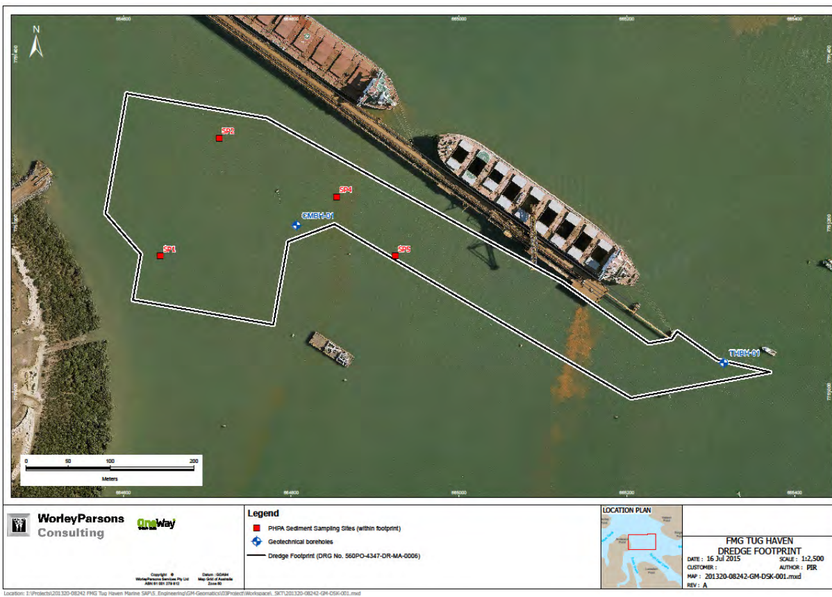
Figure 2-1: Locations of previous samples within the proposed dredge footprint
