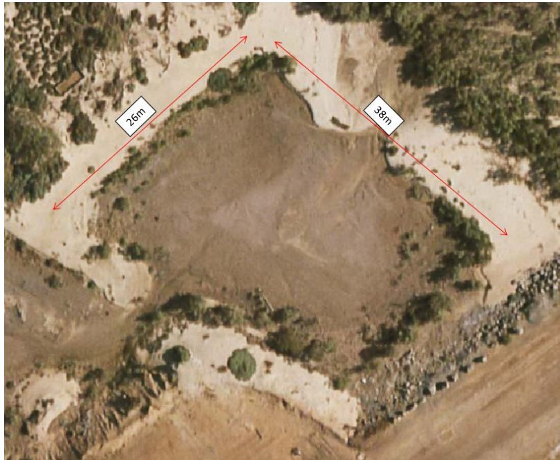
Figure 7-1 Approximate sedimentation basin dimensions (ArcMap 2015)
