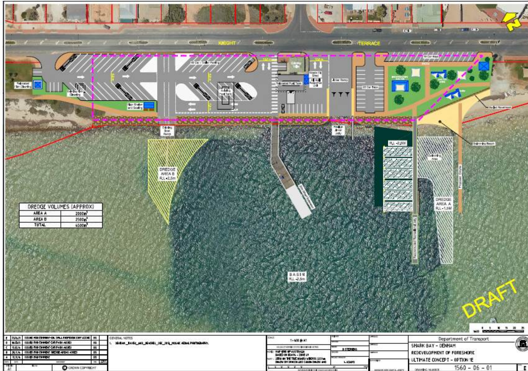
Figure 2-3 Concept plan for Denham foreshore and marine facilities upgrade. Note that the plan also includes the new recreational jetty (Stage 1) and maintenance dredging areas.
