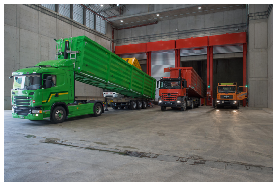
Figure 8: Waste trucks discharging their load into waste bunker in a WtE plant.
