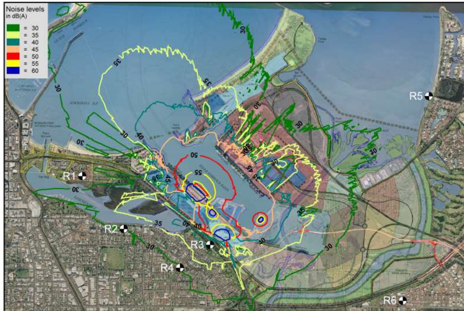
Figure C14. Worst-case night-time noise level contours for operating scenario 3c.
