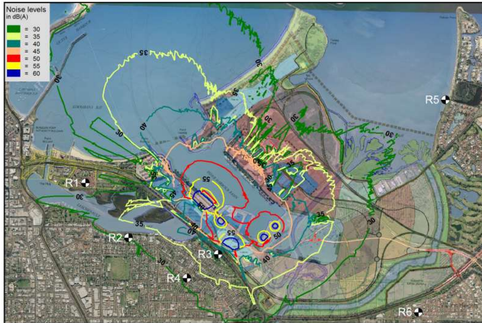
Figure C9. Worst-case day-time noise level contours for operating scenario 3a.
