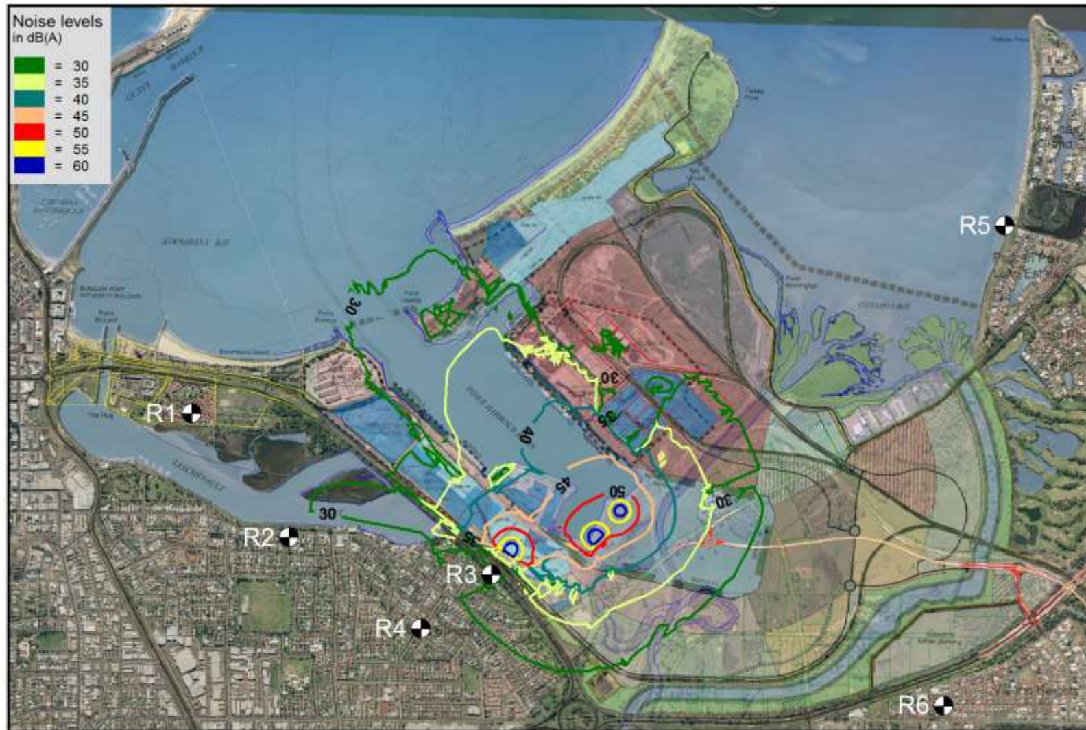
Figure C2. Worst-case night-time noise level contours for operating scenario 1a.
