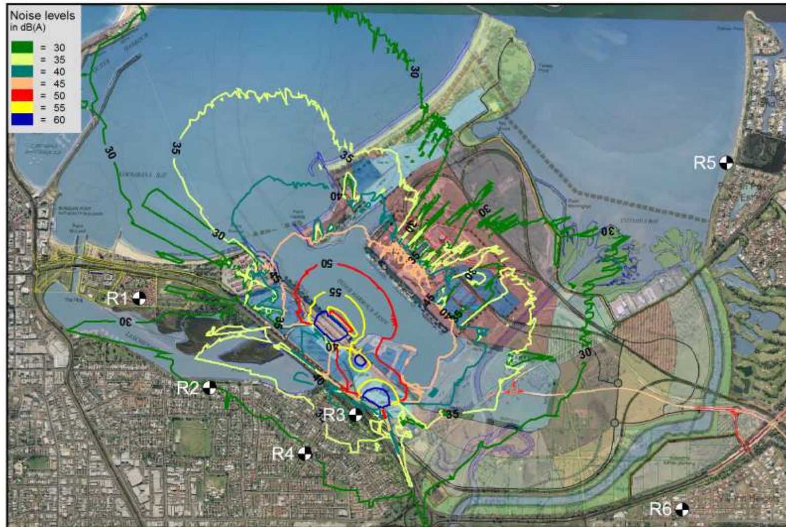
Figure C7. Worst-case day-time noise level contours for operating scenario 2.
