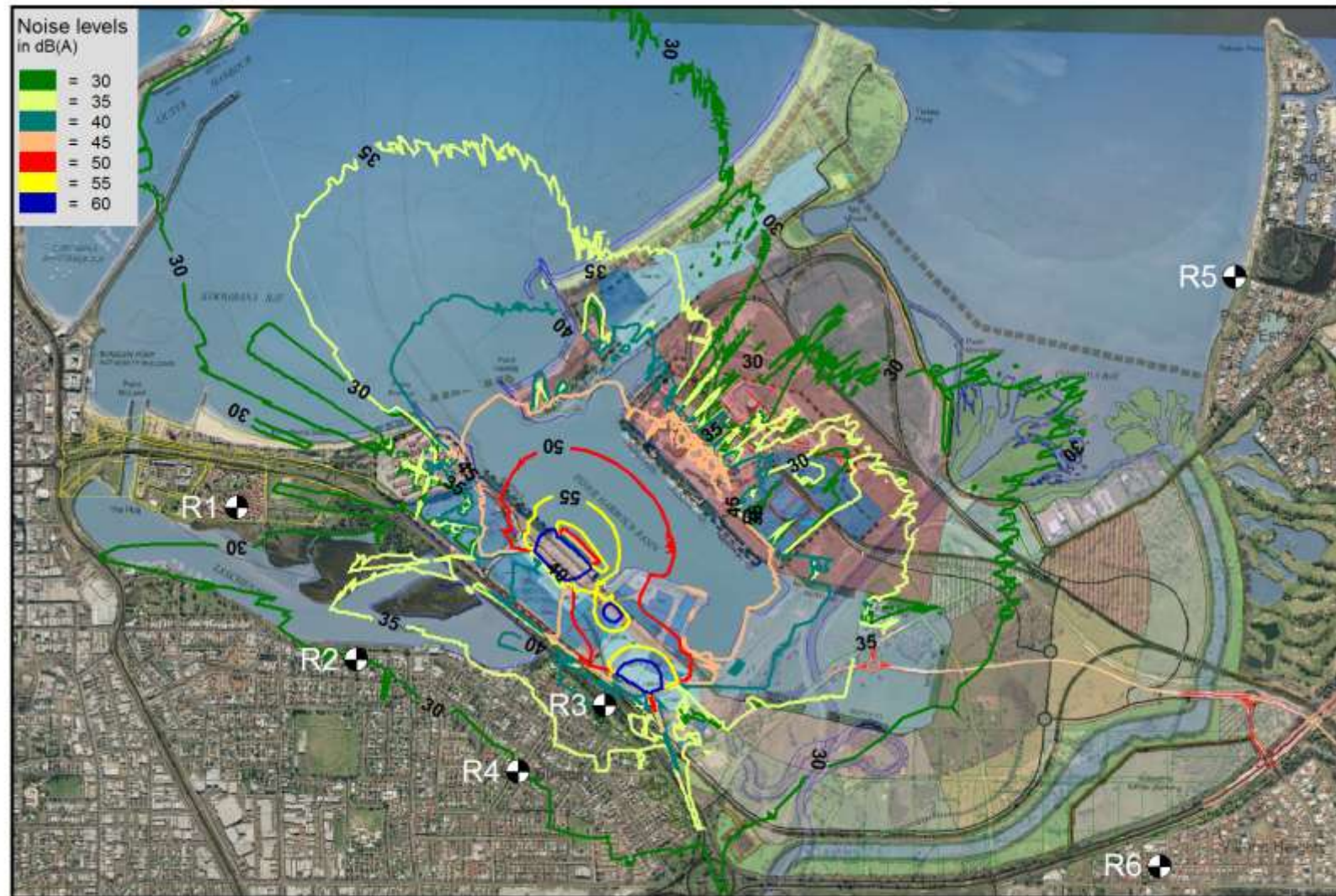
Figure C8. Worst-case night-time noise level contours for operating scenario 2.
