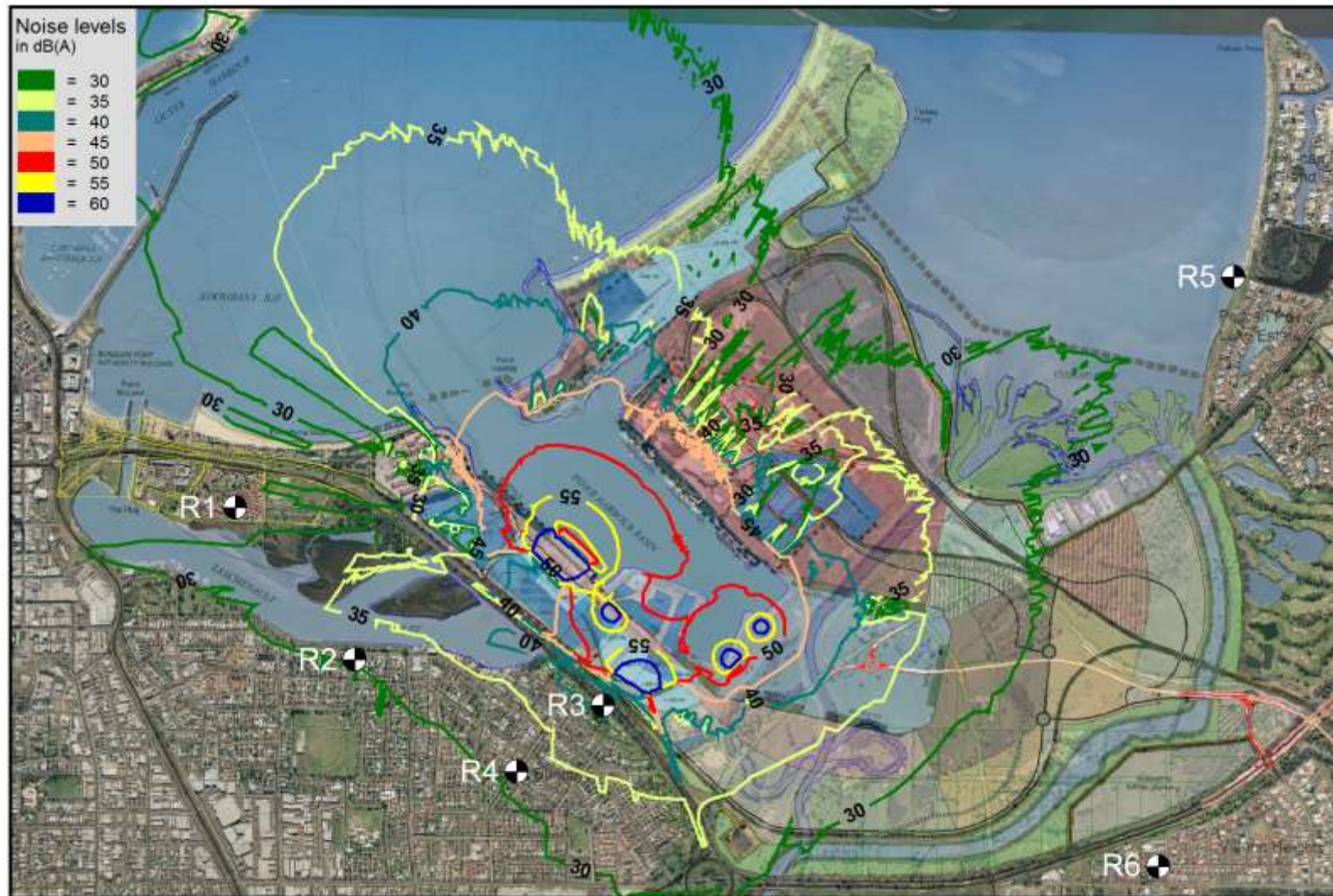
Figure C10. Worst-case night-time noise level contours for operating scenario 3a.
