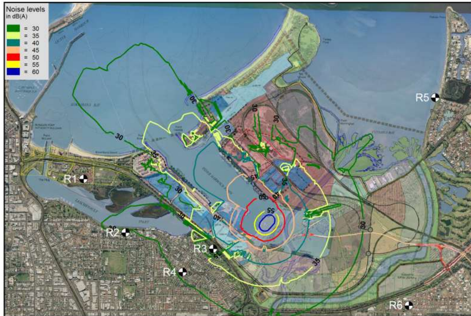
Figure C4. Worst-case night-time noise level contours for operating scenario 1b.
