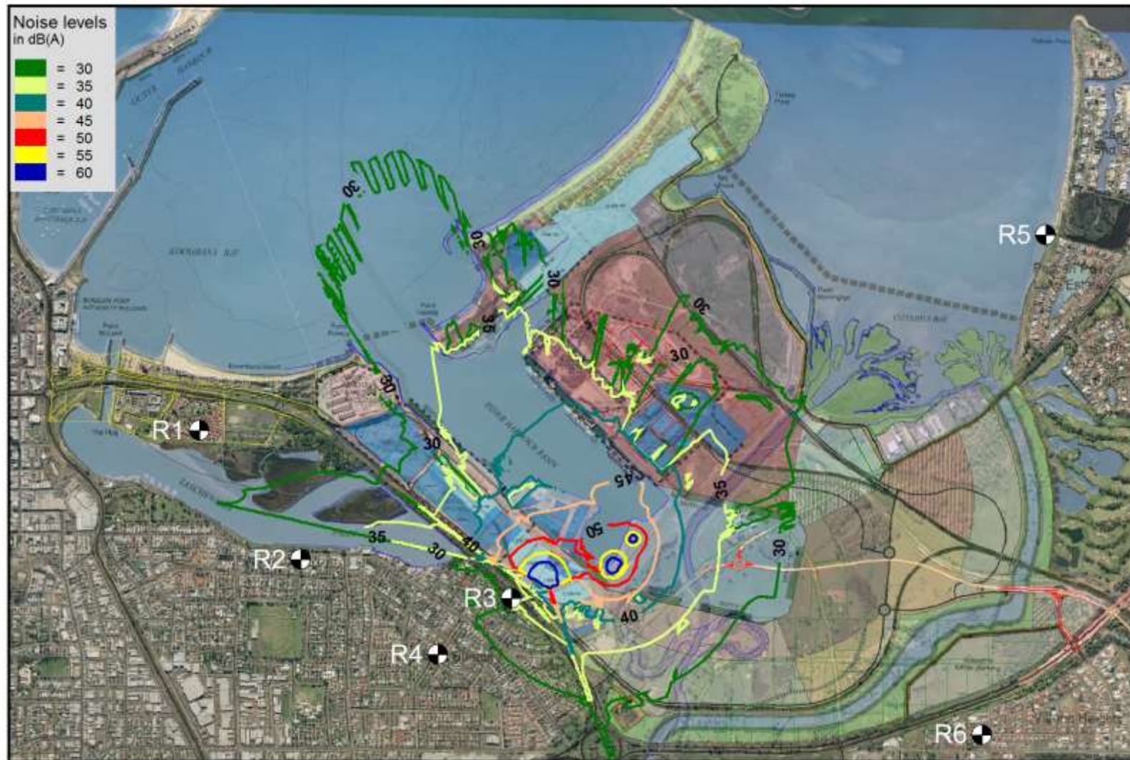
Figure C5. Worst-case day-time noise level contours for operating scenario 1c.
