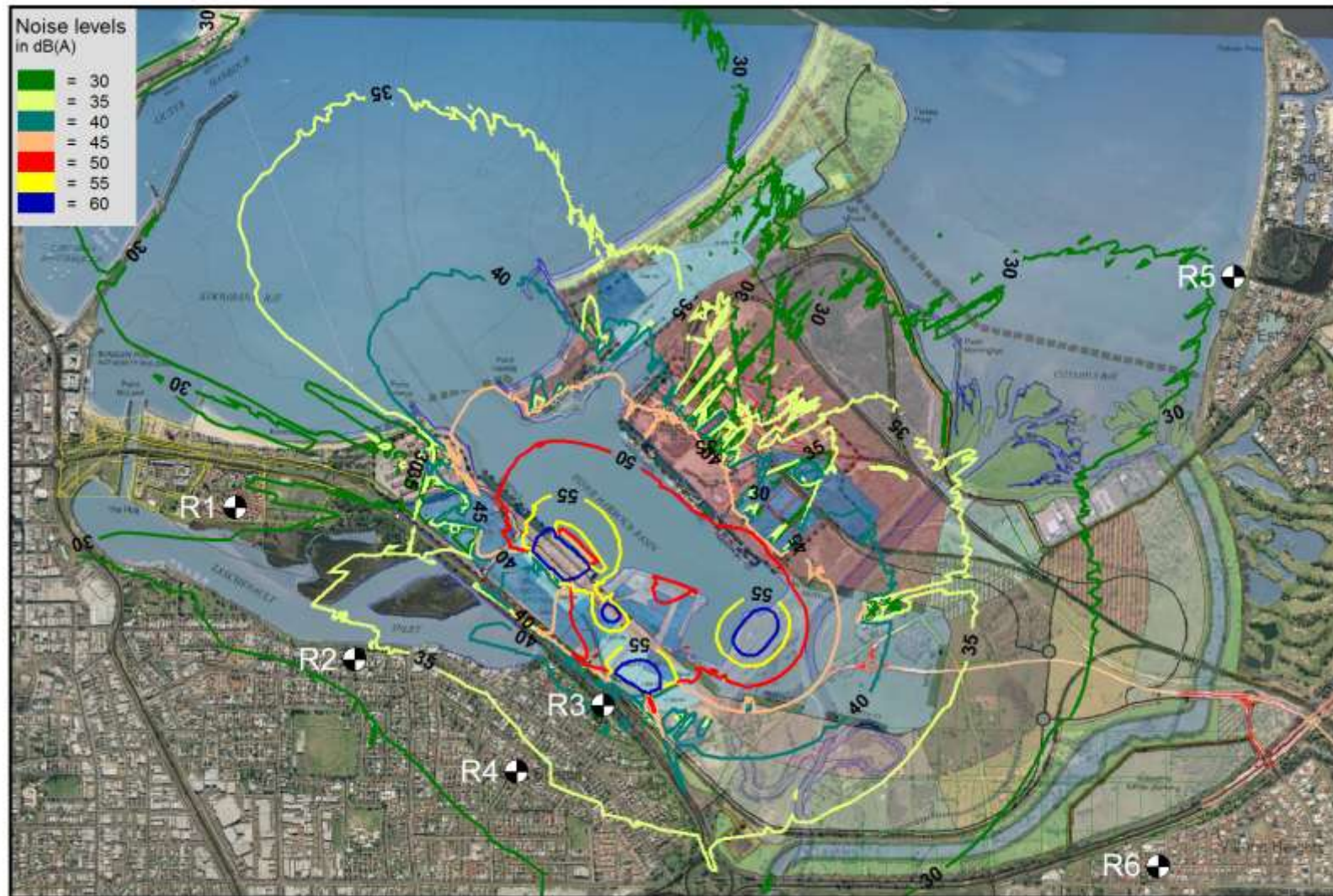
Figure C12. Worst-case night-time noise level contours for operating scenario 3b.
