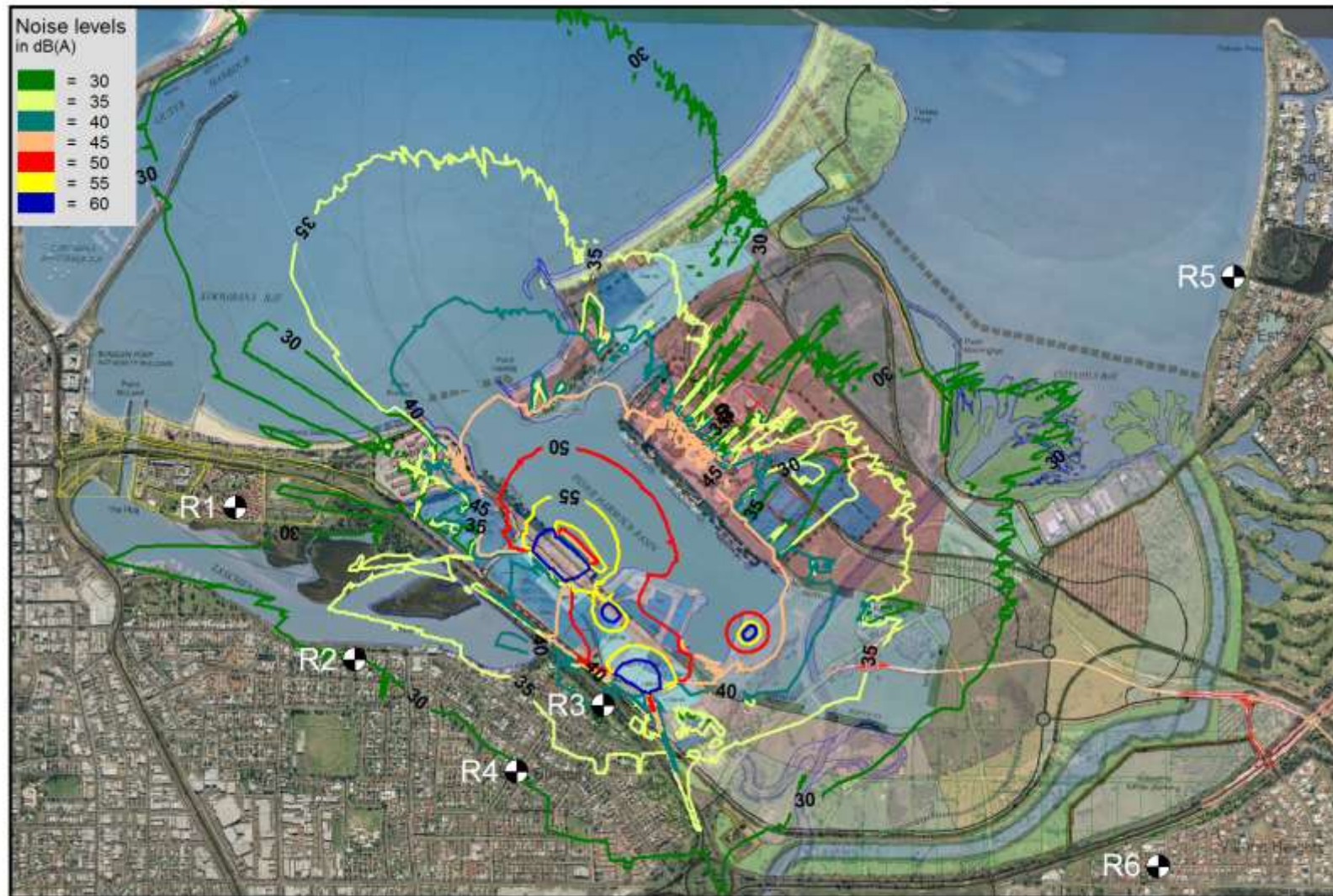
Figure C13. Worst-case day-time noise level contours for operating scenario 3c.
