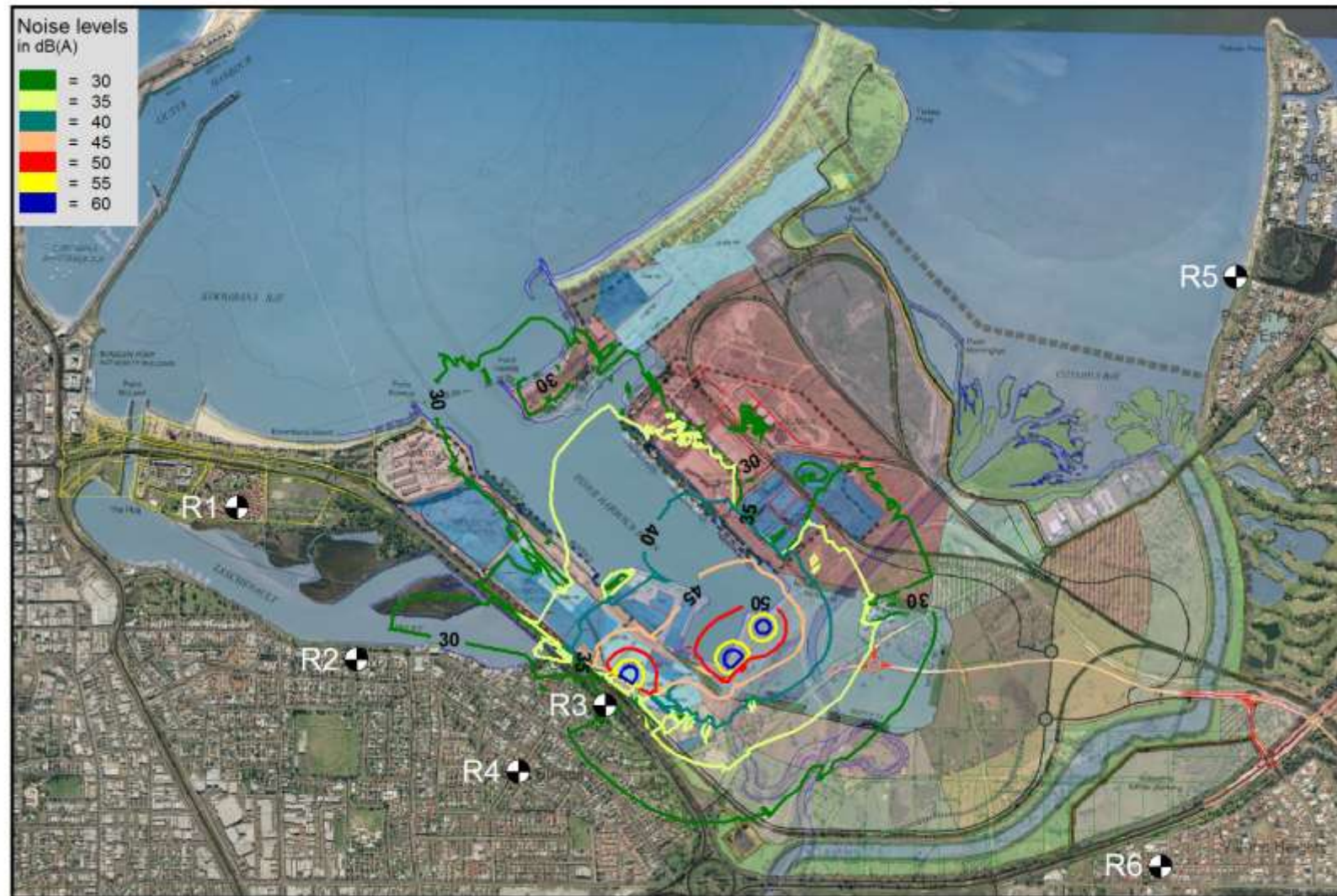
Figure C1. Worst-case day-time noise level contours for operating scenario 1a.
