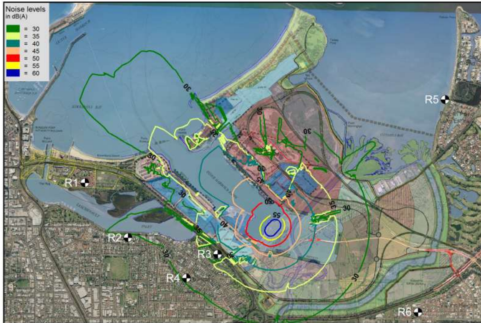
Figure C3. Worst-case day-time noise level contours for operating scenario 1b.
