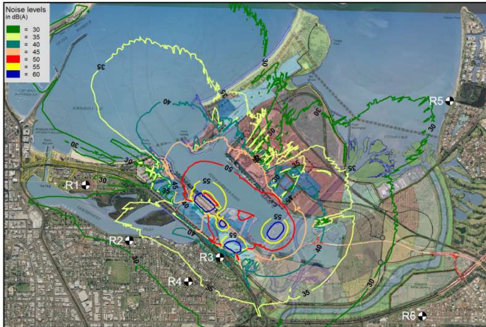
Figure C11. Worst-case day-time noise level contours for operating scenario 3b.
