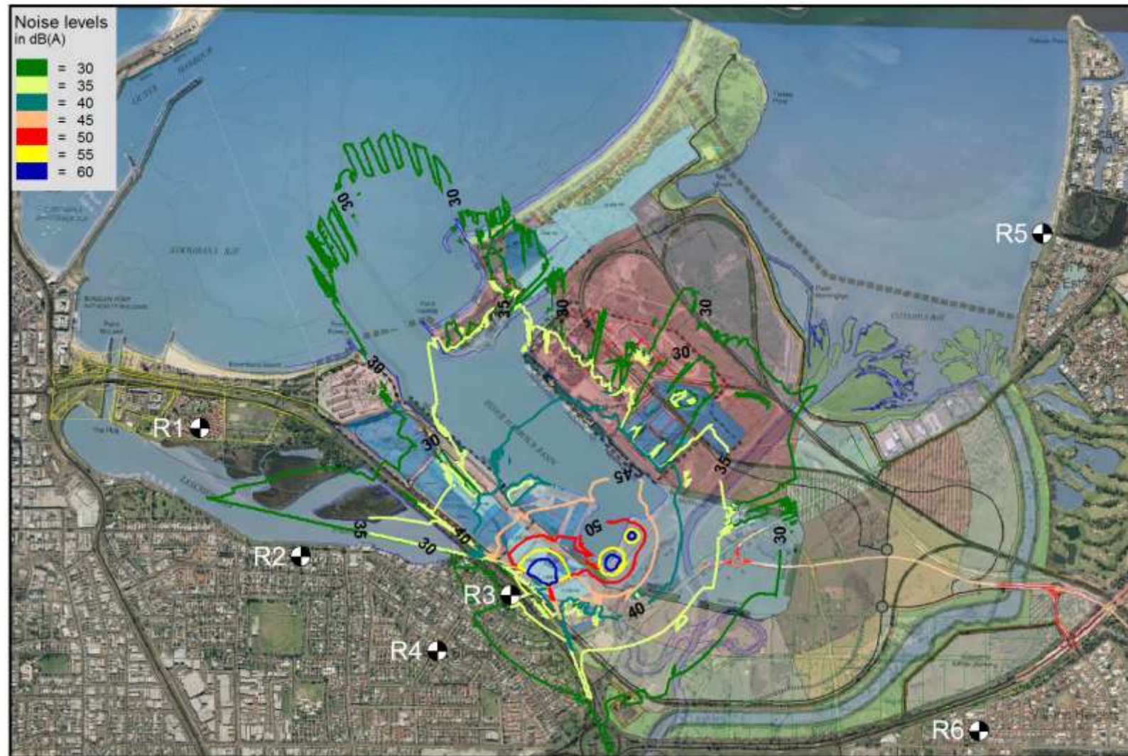
Figure C6. Worst-case night-time noise level contours for operating scenario 1c.
