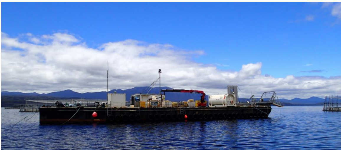
Figure 14 – Accommodation and service barge
