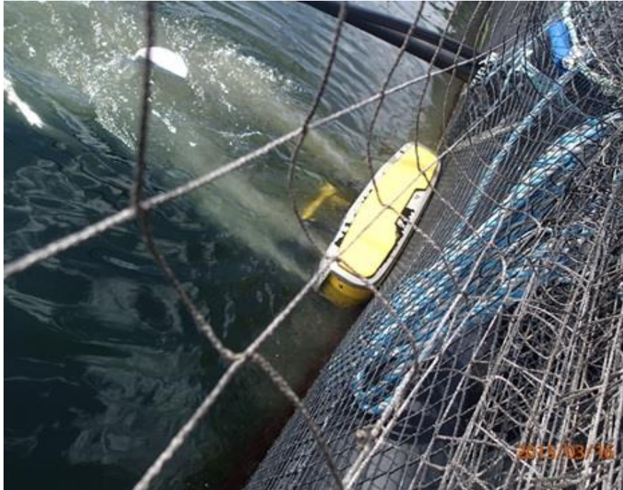
Figure 12 – RONC net cleaner in operation, note retro-jets holding the unit against the net
