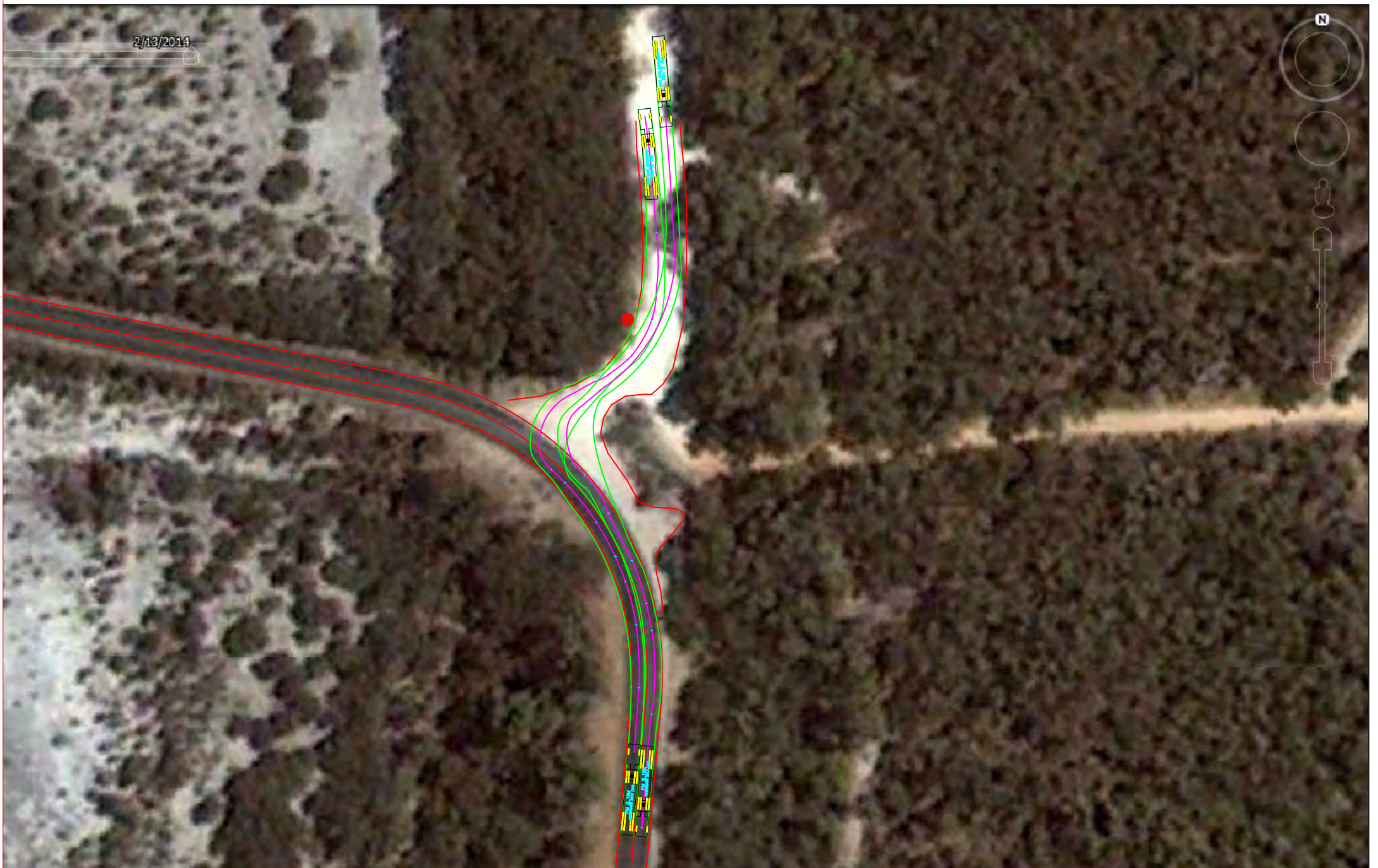
DESIGN VEHICLE 19M SEMI-TRAILER PLAN SHOWING TEMPLATES FOR RIGHT TURN-IN LEFT TURN-OUT
