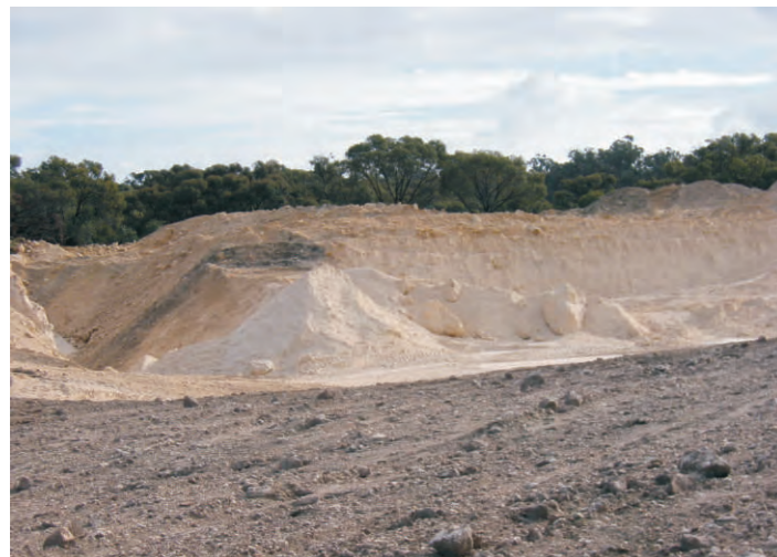
Typical crushed lime resource showing working behind a face as proposed
