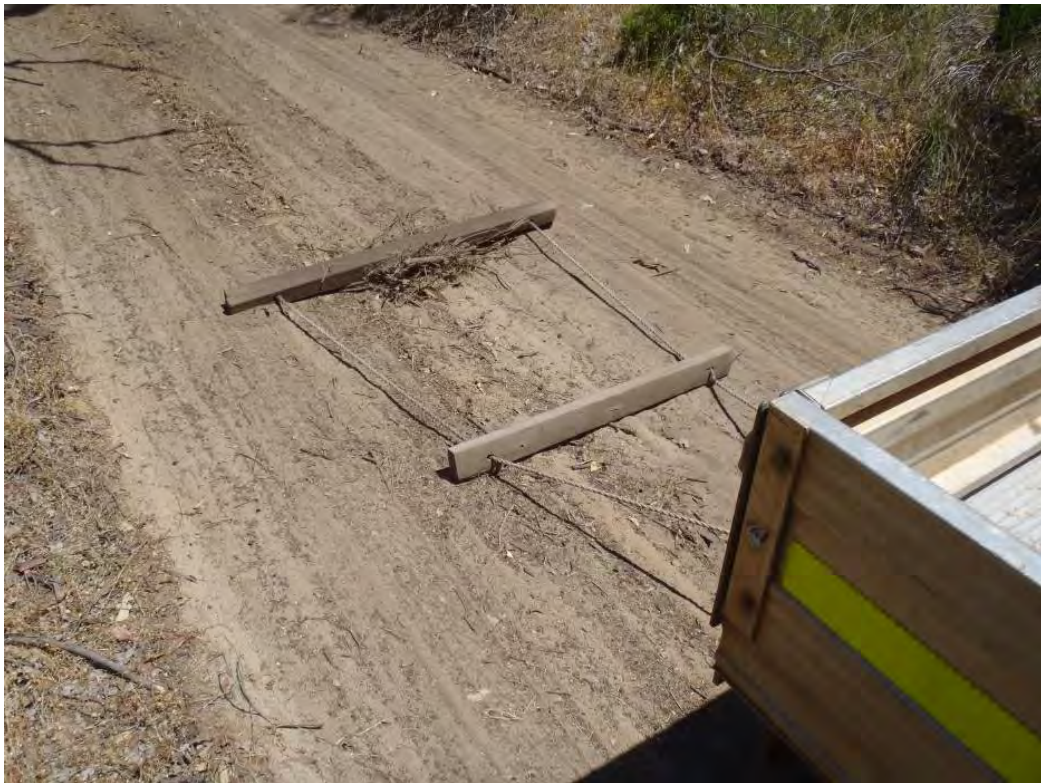
Plate 1 Wooden drag structure (without branches attached)
