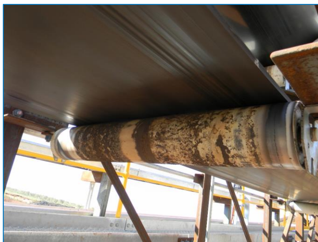
Figure 3-2: Material adhering to return conveyor
