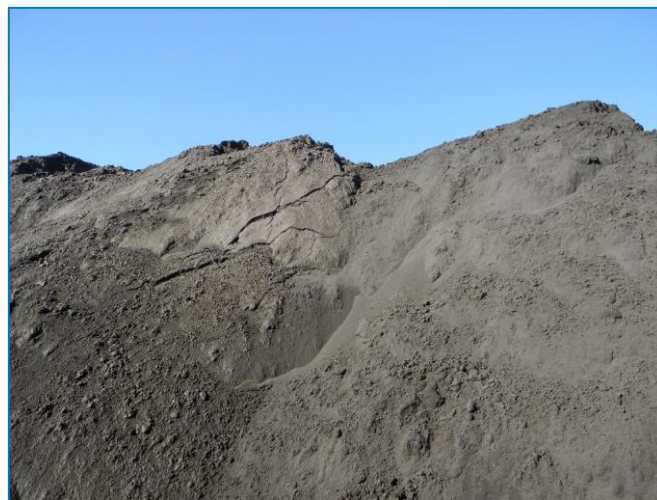
Figure 3-8: Crust and wet/dry spots on stockpile
