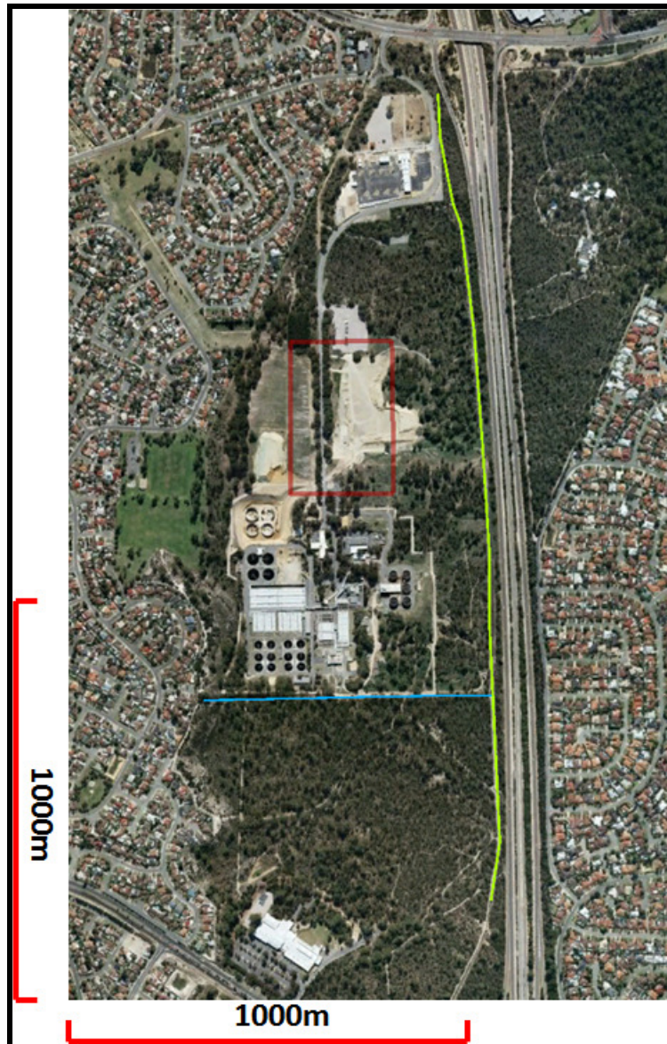
Figure C.2 - Location and position of both 2D transects over the Beenyup site. The blue line is the East – West Transect and the green line is the North South Transect. The transparent red box is the approximate extent of the 3D seismic survey.
