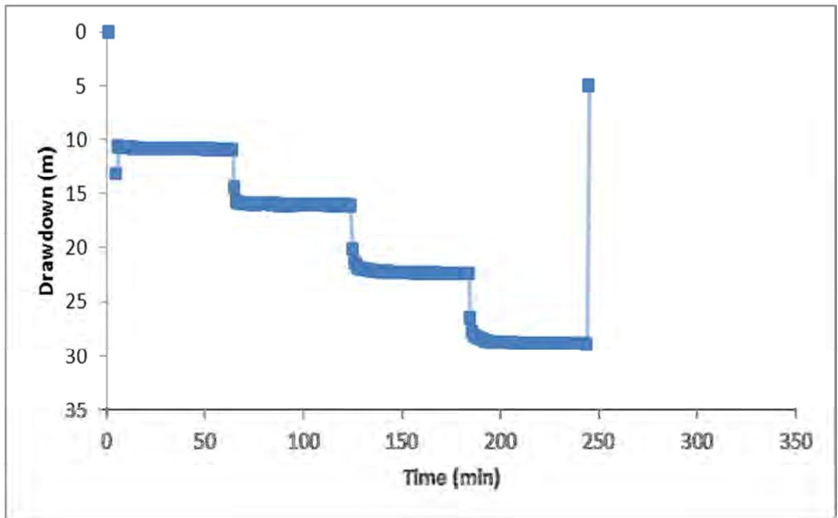
**Figure 5-9: Drawdown and Recovery at Champion Production Bore during Step-Discharge Test**
