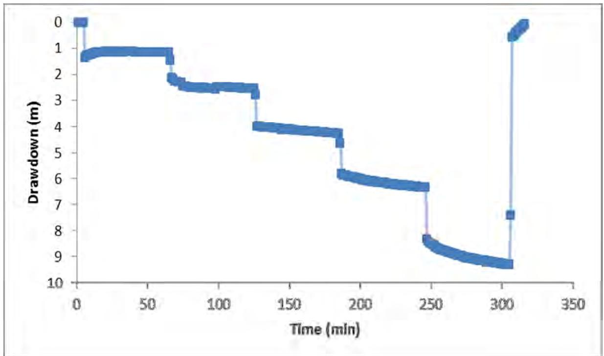
**Figure 5-8: Drawdown and Recovery at Eagle Production Bore During Step-Discharge Test**
