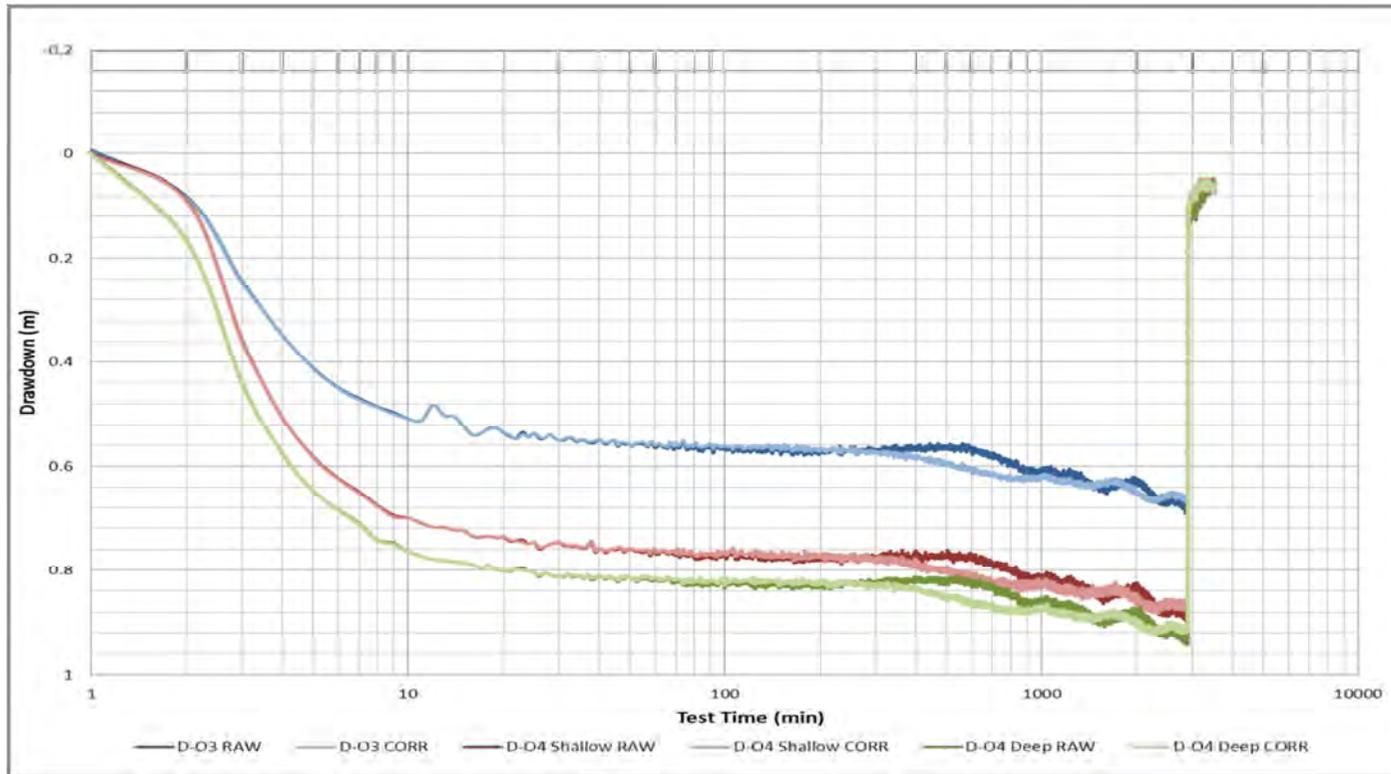
**Figure 5-5: Delta Corrected and Uncorrected Drawdown Data**
