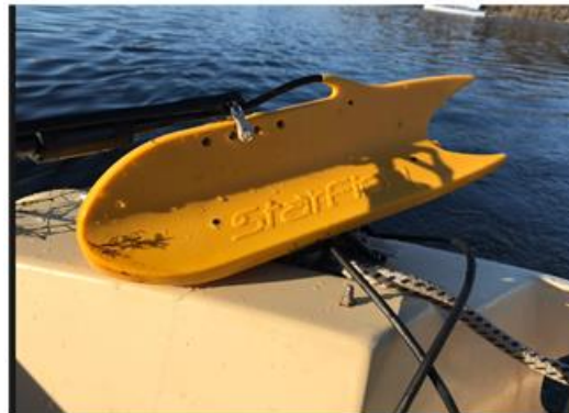
Figure 3-3 Survey Equipment a) Spot X drop camera b) Starfish 450 Khz side scan sonar
