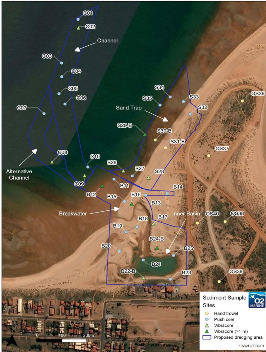
**Figure 5.1: Sediment Sampling Locations commissioned by the DoT (from O2 Marine, 2019)**
