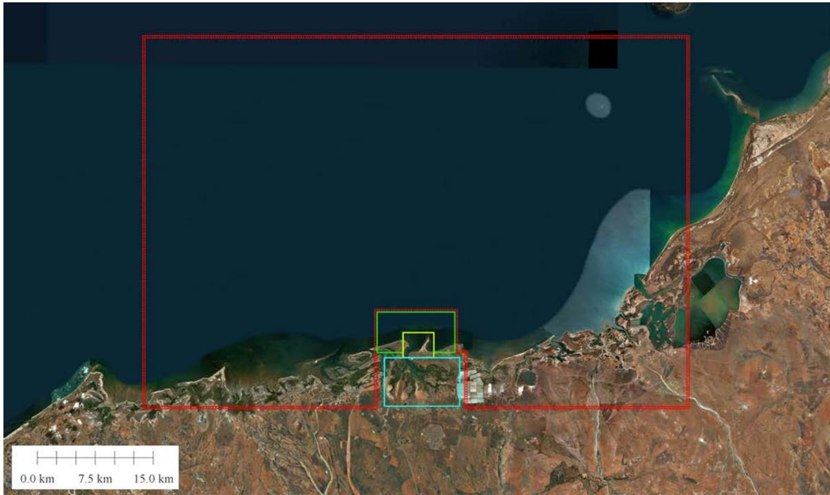
**Figure 3.12: Local Delft3D Flow-Wave-Flow Model Layout. Outer grid (red) is 315m resolution, Nearshore grid (green) is 45m resolution, Local grid (yellow) is 5m resolution and the Inner Harbour grid (blue) is 45m resolution.**
