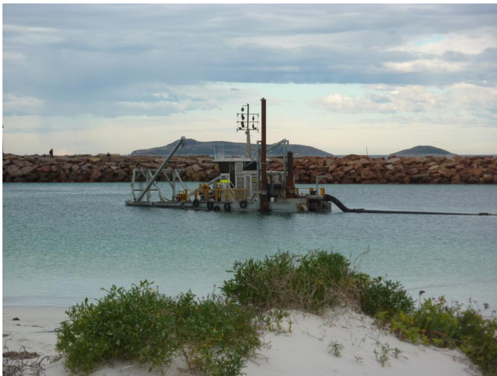
Figure 2.2 Cutter-suction dredge at Bandy Creek Boat Harbour
