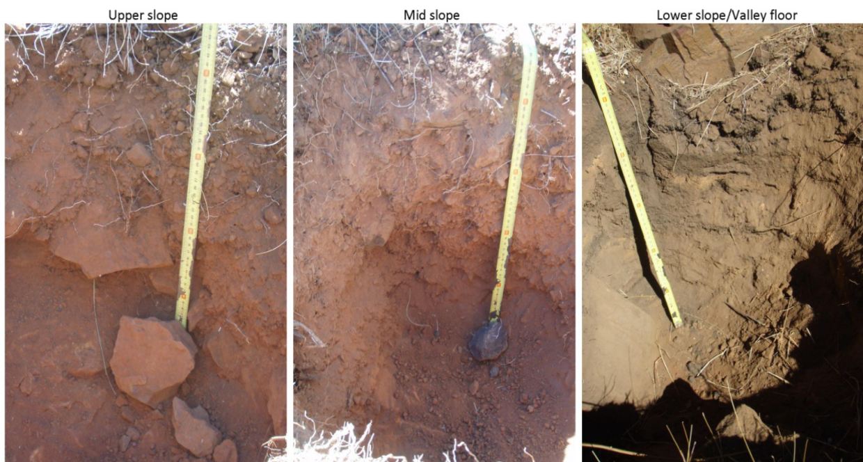
Plate 4.2: Nature of the surficial soils in SMU 1 with distance downslope.
