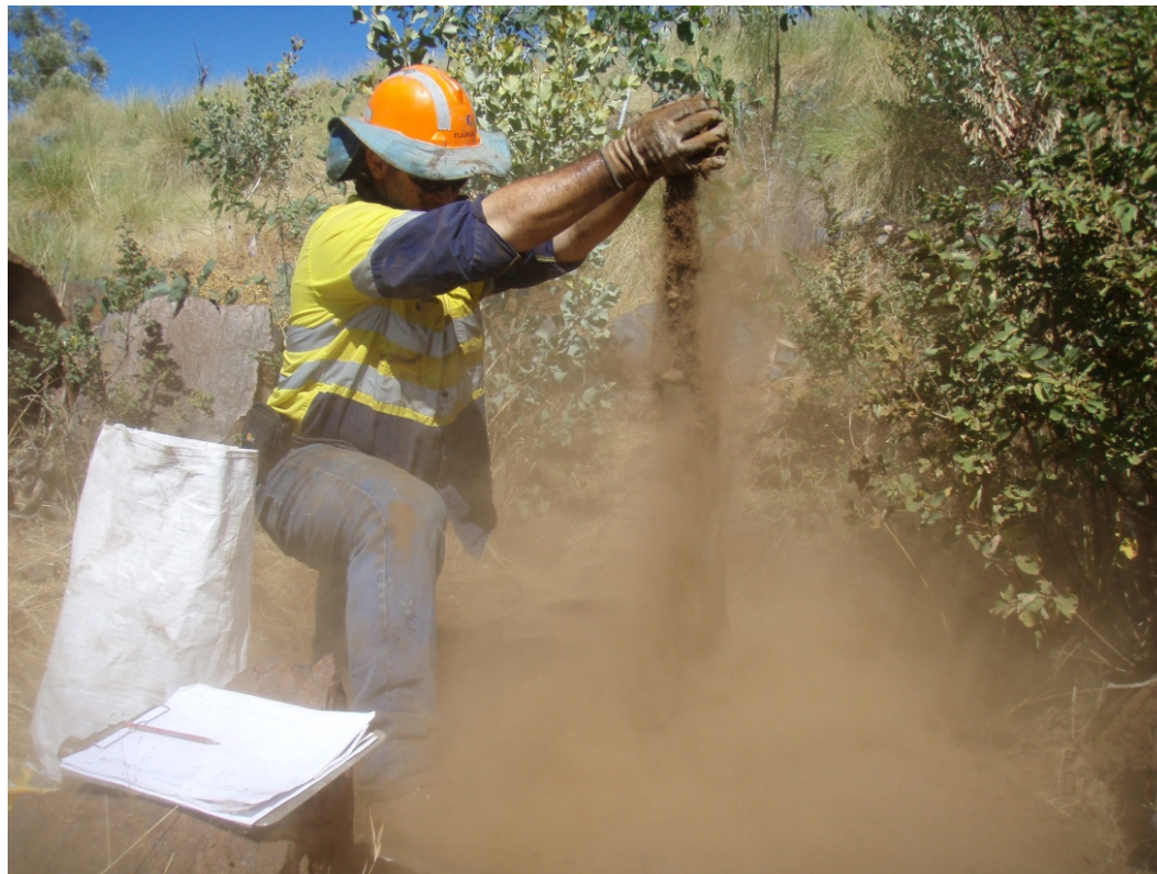
Plate 4.4: High wind erosion potential of the surface soils in SMU 1.
