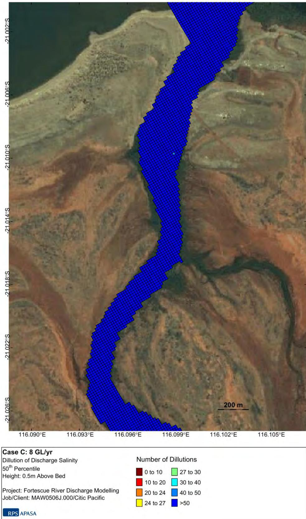
Figure 5-13: Median dilution result for Case C (8 GL/yr) at a height 0.5 m above the river bed
