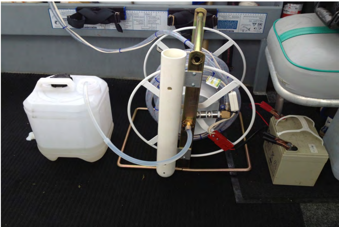
Plate 2: 12v Surface Water Pump (18 December 2012)
