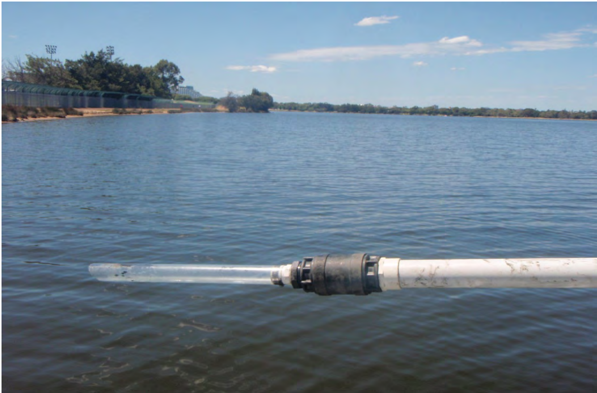
Plate 1: Sediment Corer with One Way Valve and Extension (11 December 2012)
