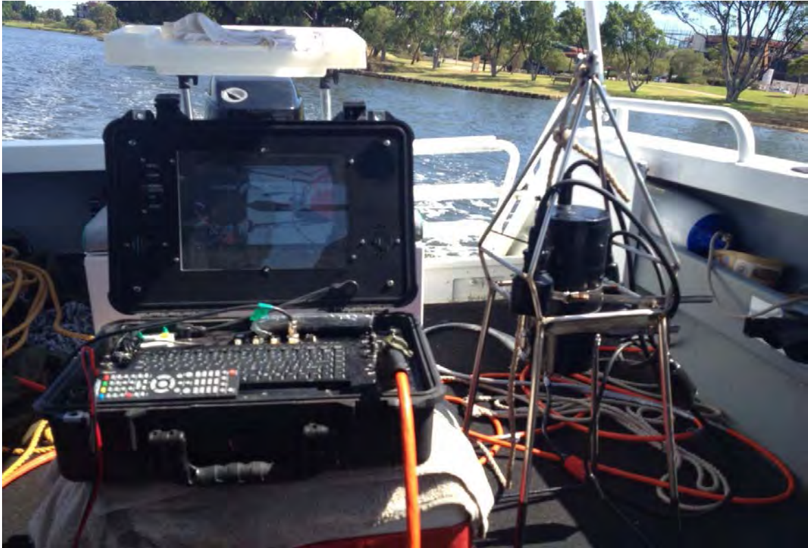
Plate 3: Drop Camera with On-board Viewing Monitor (7 January 2013)
