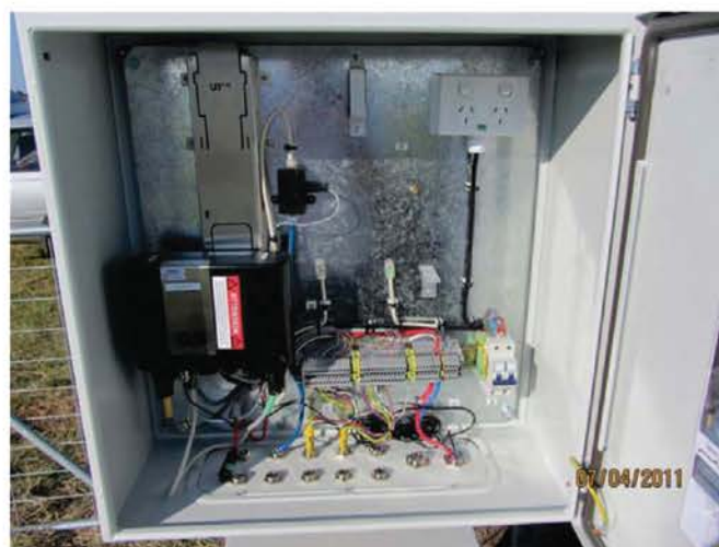
2.3 Inside the housing showing electronics for data collection
