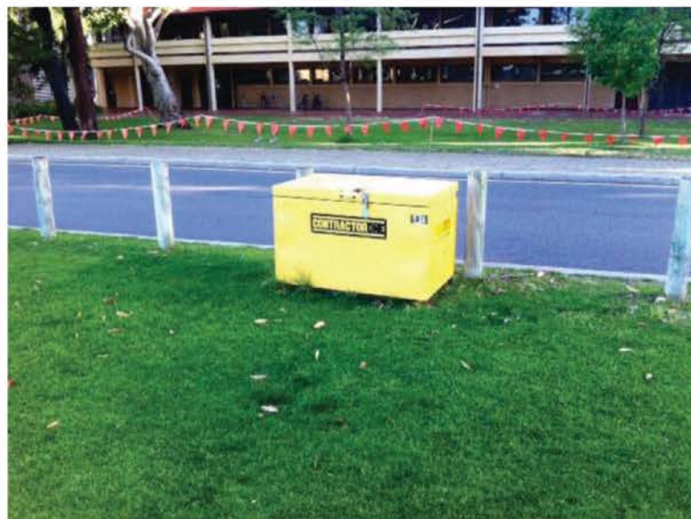
1.2 Example electronics housing (box) with mains power (on UWA campus). Broadband sensors are buried at 1m depth below surface.
