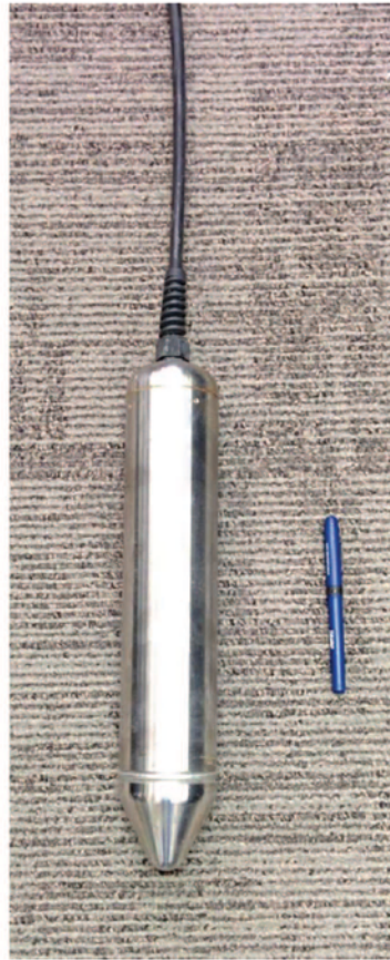
2.4 Example of seismic sensor (sonde) to be installed in borehole array
