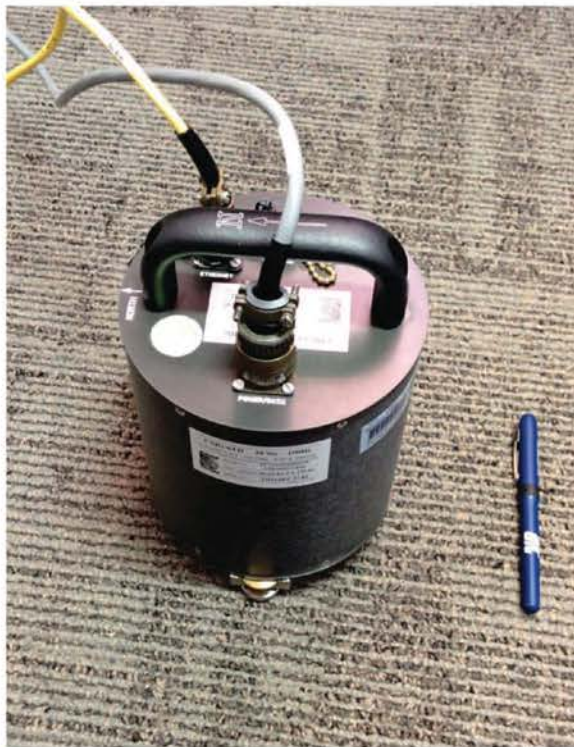
1.4 Example broadband sensor (0.03-100 Hz) installed in 1m pit
