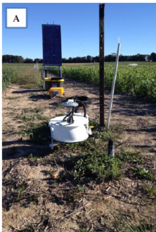
Fig 2 A. Long-term soil gas flux measurement chamber; B Soil Collar (PVC pipe (dimensions: internal diameter 20 cm; height 12 cm; thickness 0.6 cm) will be inserted into the surface soil to a depth of about 3-4 cm.
