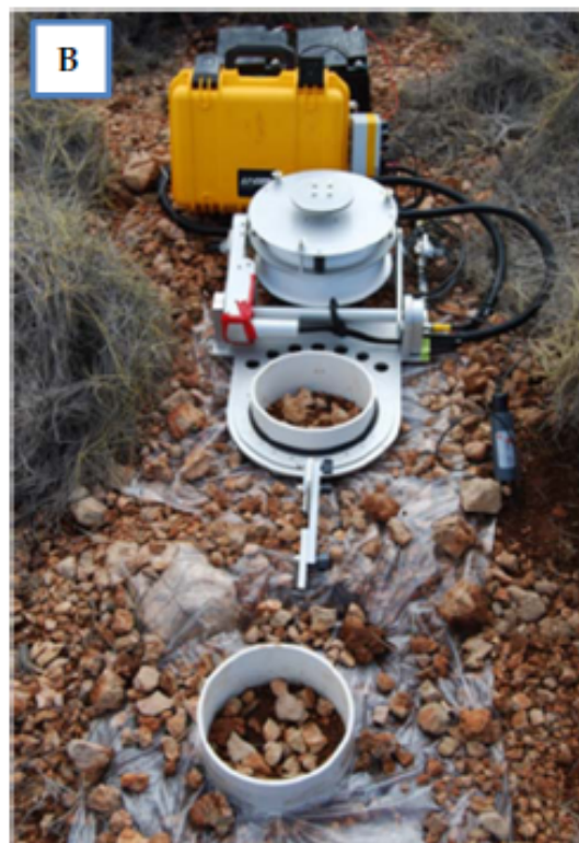
Fig 2 A. Long-term soil gas flux measurement chamber; B Soil Collar (PVC pipe (dimensions: internal diameter 20 cm; height 12 cm; thickness 0.6 cm) will be inserted into the surface soil to a depth of about 3-4 cm.
