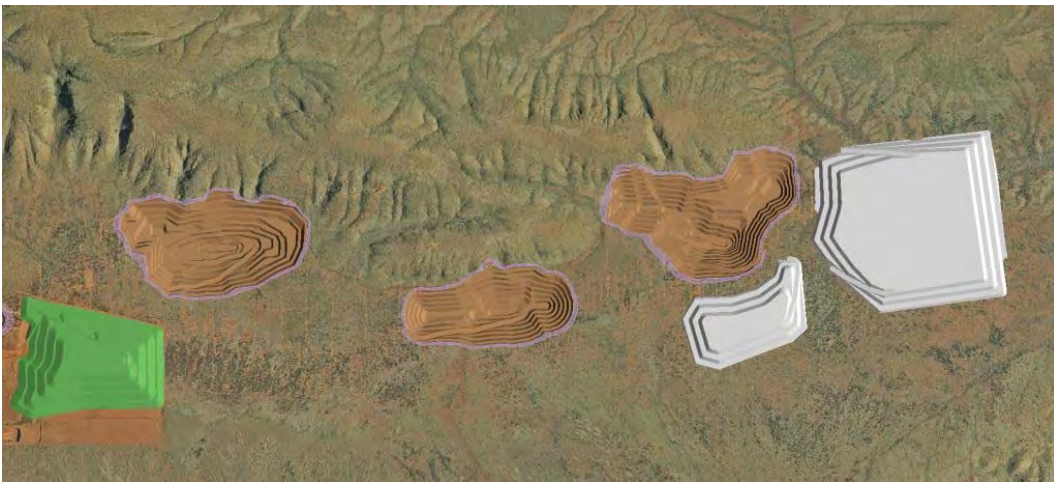
Figure 12: Zone of geotechnical instability around Deposit F
