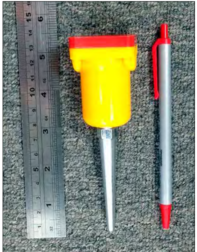
Plate 3.2 Example of a true cable free node
